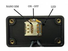
The device is intended for listening to conversations from a room over very long distances. The device operates on the principle of GSM network, and for its normal operation it is necessary to ensure a normall SIM card. The location where the device will operate must be covered by a GSM signal (check with a regular cell phone).
