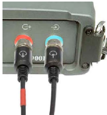
Fig.16 HF-cables coupling to the Main unit
