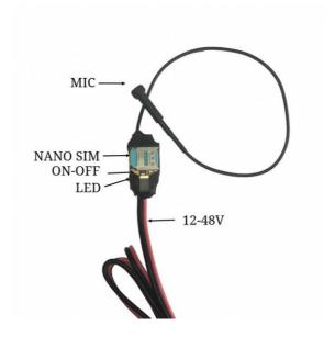
**NOTES:** The device is intended for listening to conversations from a room or car over very long distances. The device works on the principle of GSM network, and for normal operation it needs to provide a 2G SIM card. The place where the device will work must be covered by a GSM signal (check with a regular mobile phone).
