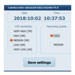
Here you can change the parameters of the voice activation sensitivity, recording quality and synchronize the date and time on future recordings.
