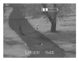
Transmitting channel generates laser beam in the form of vertically located rectangular raster. Ability of illuminating raster can be changed if necessary, depending on distance to surveillance object, for reception of the best image contrast. Image focusing on sharpness is carried out by adjustment of video camera objective.
